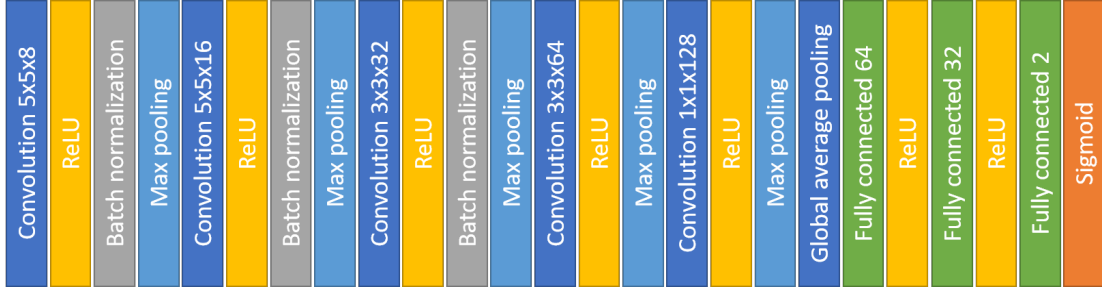
Figure 4.2: Architecture of the neural network devised to estimate distortion parameters, named DPEN
