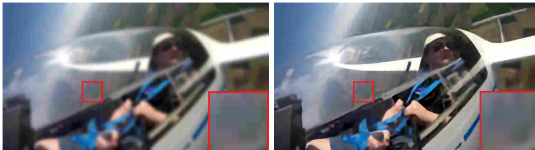
Figure 5.8: Example of a multi-distorted frame (left) affected by Gaussian blur ( \sigma = 4 ) and JPEG compression artifacts ( q = 15 ) restored by FastDVDNet [28] (right)
