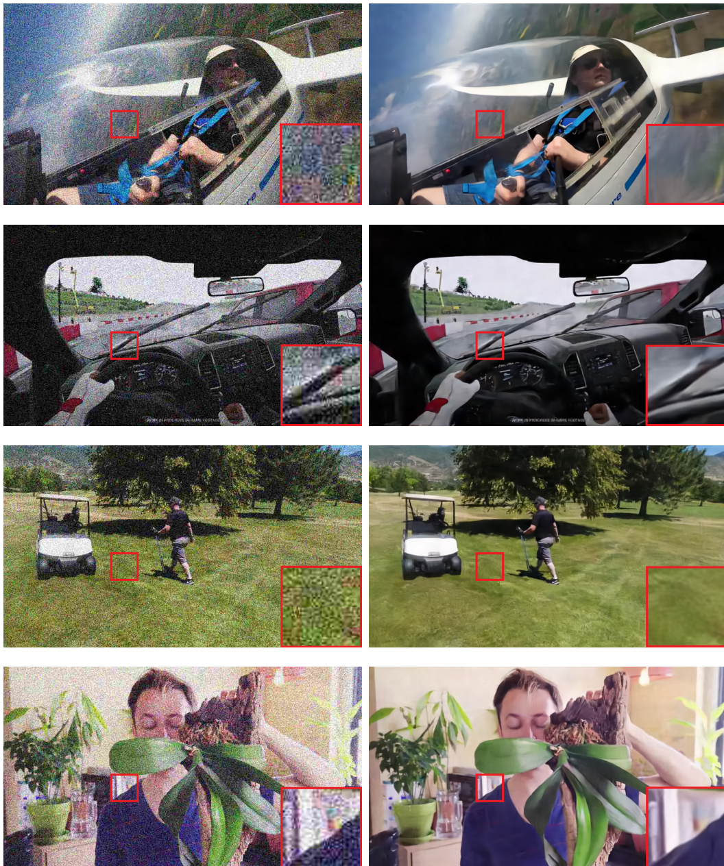
Figure 5.10: Qualitative results of MdVRNet in restoring videos simultaneously affected by additive white Gaussian noise ( \sigma = 50 ) and JPEG compression artifacts ( q = 15 ). Distorted frames on the left, restored frames on the right.
